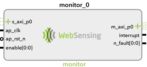
A Software Monitor block that continuously monitors the integrity of software to detect malicious, zero-day implants. This block can be hidden within an SoC on-chip FPGA hardware to monitor the Linux Kernel, device drivers, and/or applications running on the SoC processors.
