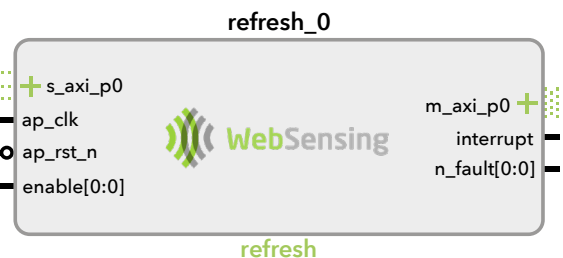
A Software Refresh block capable of restoring software to a "gold-standard" image thereby removing malicious implants.
