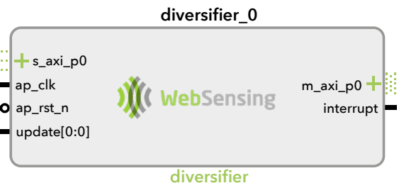
A Software Diversifier block capable of loading "diversified" software images thereby preventing re-infection. The images can be generated from source code using our compiler transformations.
