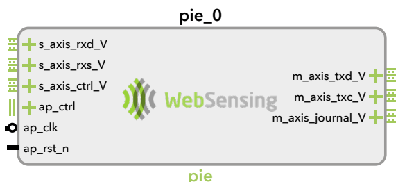
A Software Barrier block for isolating software memory regions and processes thereby providing cross-domain protections.
